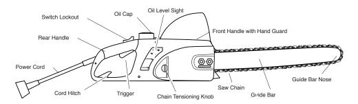
Figure 3 - Chain Saw Model 107625-02, 111174-01
